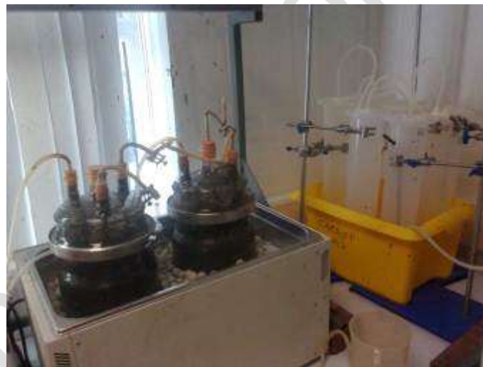
Figure 1 Bench scale plant configuration showing MAD rigs and biogas collection
